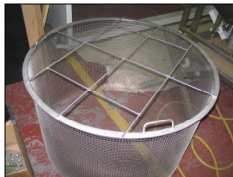
Process basket with rods for specimen hooks.
